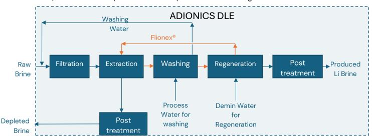
The only pre-treatment required by Adionics technology is filtration to remove solids & bio (algae...).
