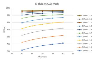
Example of a parametrical study showing the impact on yield of the amount of consumed wash water in the washing step for different O/A ratios in extraction for a given process cycle on brine 3.
