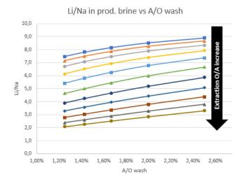
Top left graphic describes that the higher the O/A of extraction, the higher the lithium recovery yield and the lower the washing A/O ratio, the lesser the impact on the lithium recovery yield.
